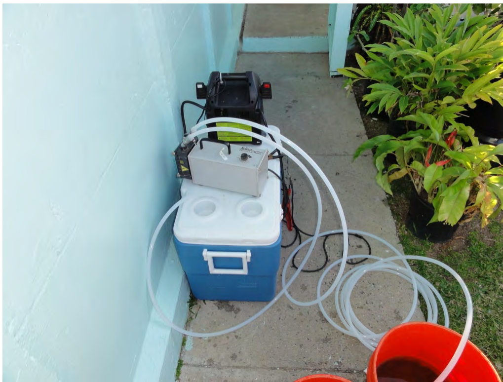
Photograph 33: Peristaltic Pump and battery pack used to vacuum the sediment.
